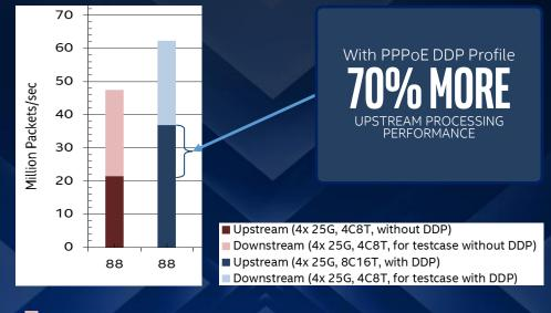
Upstream (21.42 Mpps) Downstream (25.90Mpps) with DDP Upstream (36.98Mpps) Downstream (25.18Mpps)
